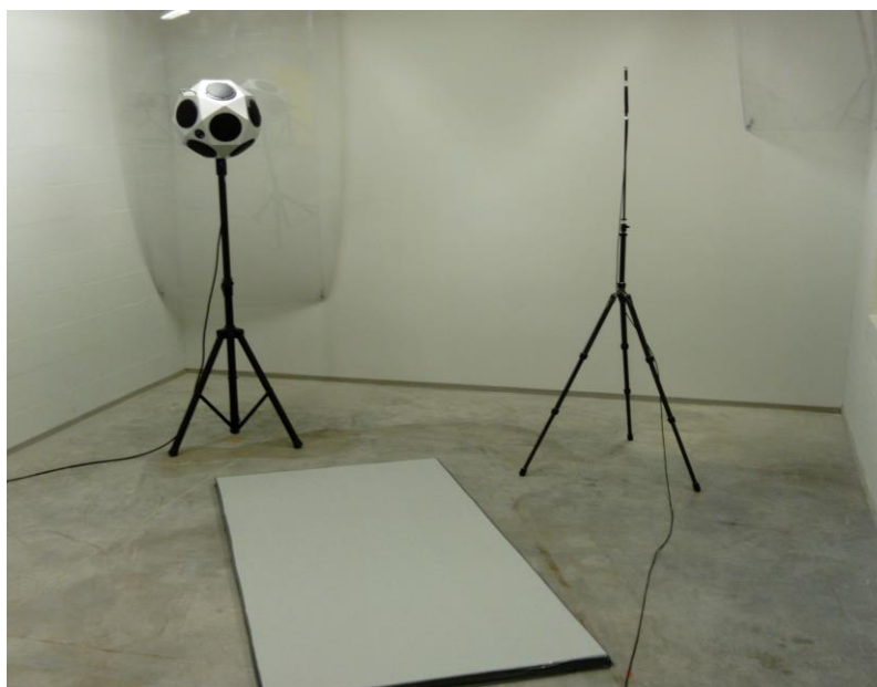
Photo A3-1. The installation of test objects (acoustic material sample) in AcouTechLab reverberation room. Omnidirectional acoustic source (loudspeaker) and tripod mounted measurement microphone are exhibited in the background.
